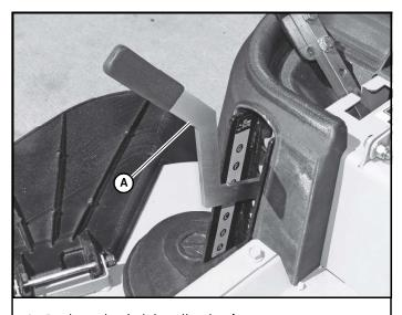
A. Deck cutting height adjusting lever
